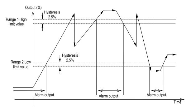
\* When an alarm output condition occurs, Digital output 1 and 2 change to the output status set for an alarm output condition. Alarm output contact is open while the converter is powered off.
